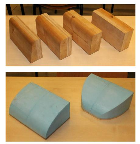
Fig. 5. Cab fronts (top) and spoilers (bottom) to be mounted using magnets
