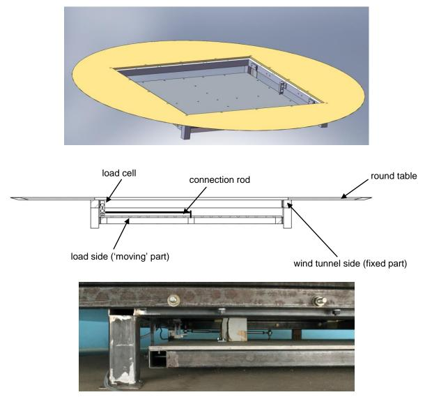
Fig. 3. The force measurement platform
