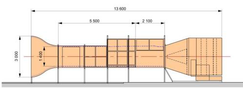
Fig. 1. The ÉMI wind tunnel
