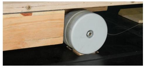
Fig. 6. Ensure that there is a gap between wheels and the cover plate, when placing the model onto the platform
